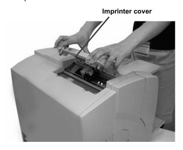
3) When the lever is closed, rotate the lever to open before placing the print cartridge.
