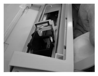
5) Lift the Upper transport unit slightly to release the safety lock and then lower and close the transport unit slowly.
